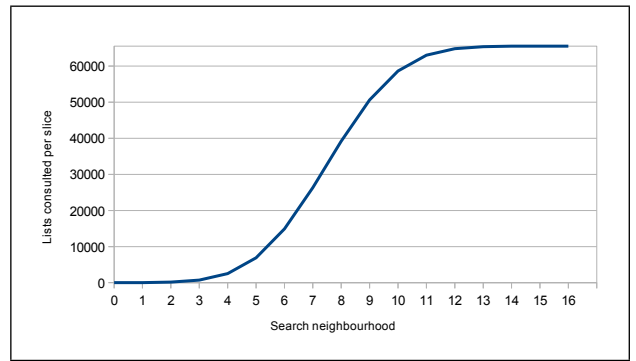
Figure 1: The relationship between the size of the search neighbourhood and the number of posting lists checked per slice. Derived from table 1.
