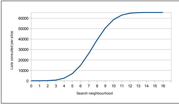
Figure 1: The relationship between the size of the search neighbourhood and the number of posting lists checked per slice
